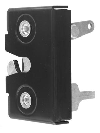
The compact 050-7200 10mm Single Rotor Latch with Dual Trip Levers is designed for operator and compartment door applications for off-highway vehicles. Offering a direct push button handle release with remote cable or rod actuated inside release providing expanded application flexibility.
